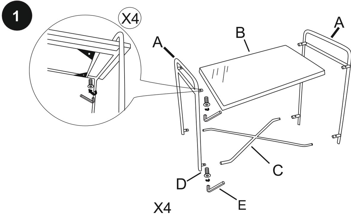
NOTE: Level the table and tighten all bolts with the allen wrench.
