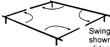
Swing out all cross rails as shown in diagram. Insert glides into legs.
